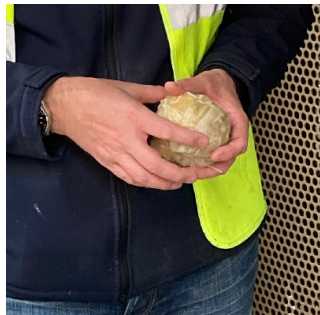
Condense the removed coating into a small ball.
